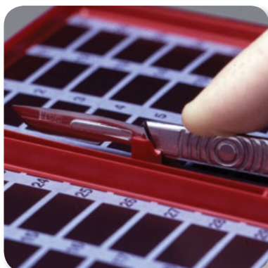
Step 2: Slide forward until blade "catches."
