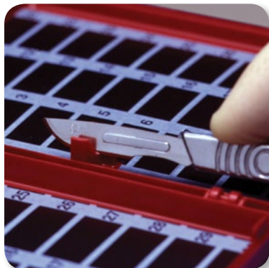
Step 1: Insert blade into DeBlade mechanism.
